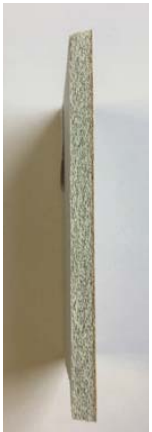
Better Shelter - polyolefin (8mm) - UV protection film
