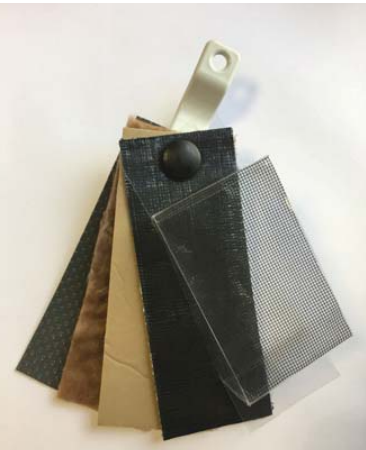
Step 5 - Altro Xpresslay (2 mm) - rockwool insulation (5 mm) - polyolefin (8 mm) - UV protection film - tarpaulin - air gap (40 mm) - black net - PET enclosure
