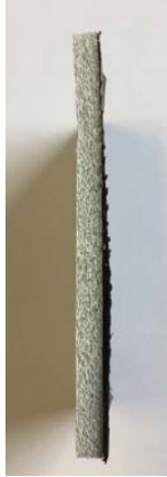
Step 1 - polyolefin (8 mm) - UV protection film - tarpaulin
