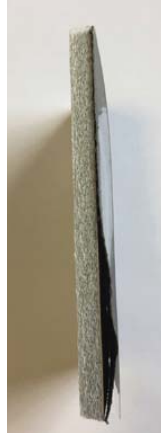
Step 2 - polyolefin (8 mm) - UV protection film - tarpaulin - PET sheet
