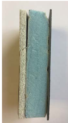
Add. Insulation #2 - polyolefin (8 mm) - UV protection film - expanded polystyrene (20 mm) - Altro Xpresslay (2 mm)
