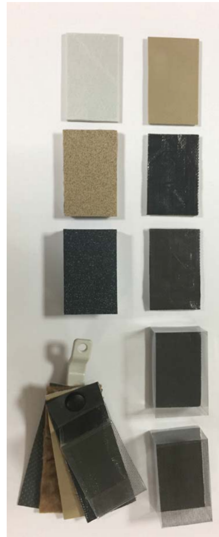
Step 4 - polyolefin (8 mm) - UV protection film - tarpaulin - air gap (40 mm) - black net - PET enclosure
