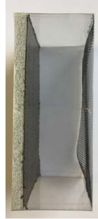
Step 4 - polyolefin (8 mm) - UV protection film - tarpaulin - air gap (40 mm) - black net - PET enclosure
