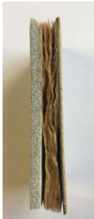
Add. Insulation #1 - polyolefin (8 mm) - UV protection film - Rockwool insulation - Altro Xpresslay (2 mm)
