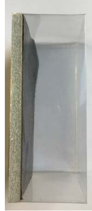
Step 3 - polyolefin (8 mm) - UV protection film - tarpaulin - air gap (40 mm) - PET enclosure
